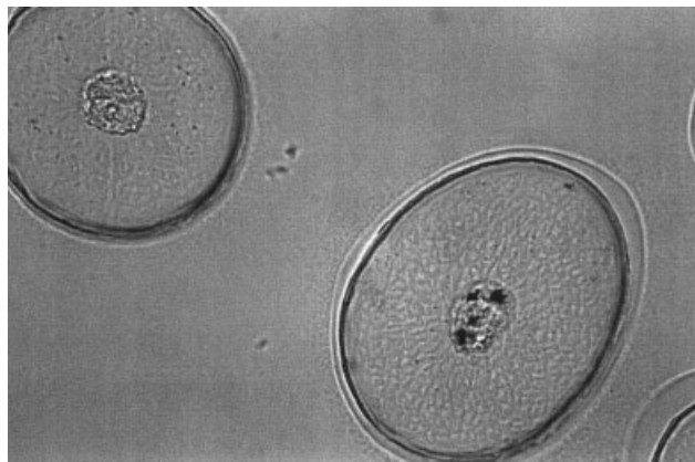
Figure 3 Cross-sectional photomicrograph of bleached white human hair dyed with Orange II, which was previously treated with 10 wt % PEI (Mw = 600) at 50°C for 15 min (sample 9).
