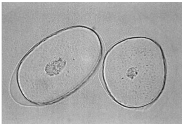
Figure 1 Cross-sectional photomicrograph of bleached white human hair dyed with Orange II, which was treated beforehand with 5.0 wt % N-methyl-2-pyrrolidone at 50°C for 15 min (sample 7).
